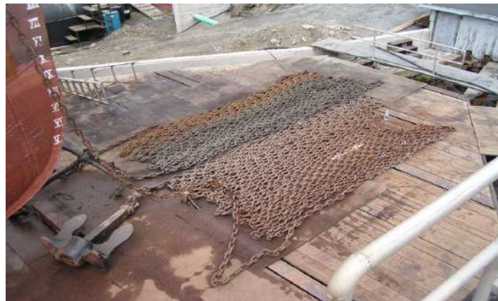
Preparing the anchor chain for marking
