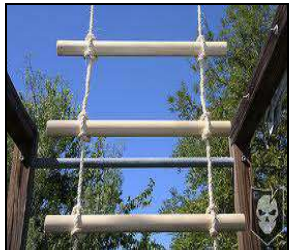
Rigged Jacobs Ladder
