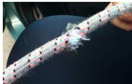
Careful inspection of the rope – shows wear/tear and rope damage
