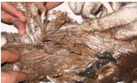
Careful inspection of the rope – shows wear/tear and rope damage
