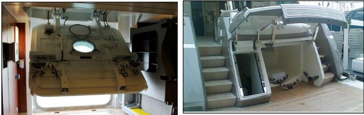
Mega yachts with watertight doors
