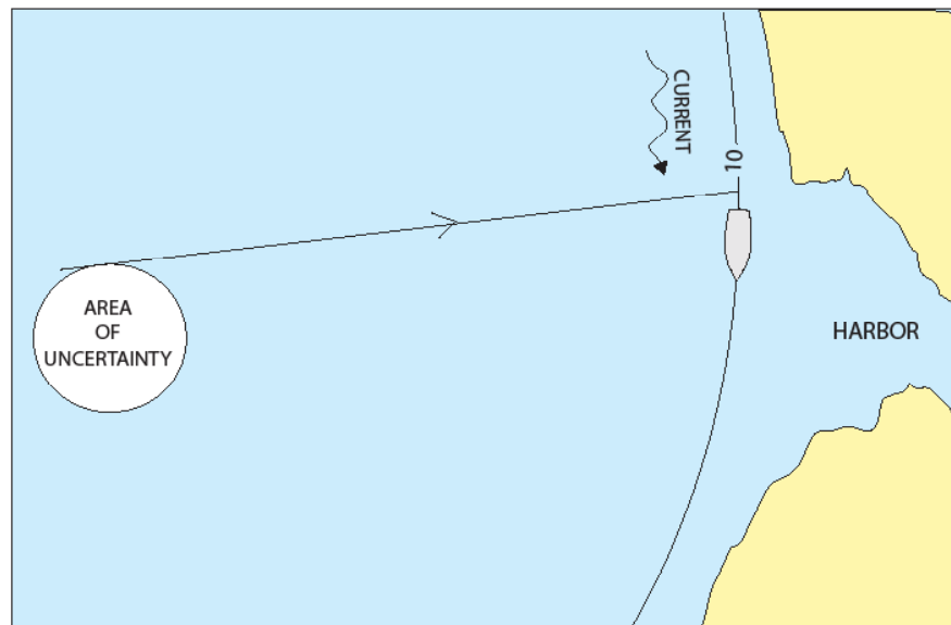
Fig. 1 The decision whether to head to the north or south of the harbour depends upon the direction of current and wind, if any.
