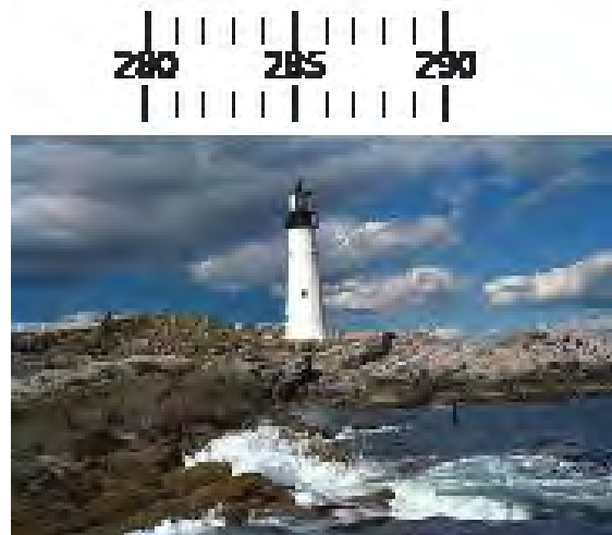
Fig 1 Taking a bearing of a light house using a hand-bearing compass. Here the bearing to the light house from your position is 285° (C)
